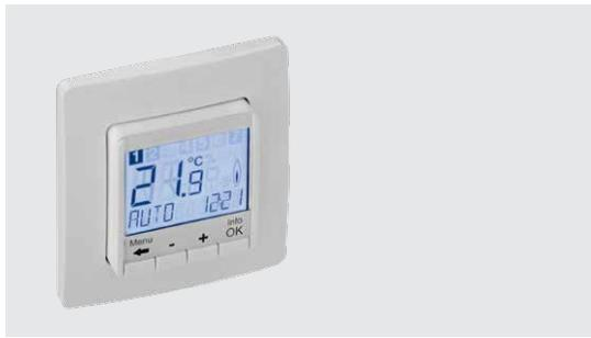
Combination of room and clock thermostat, flush-mounted, large-screen display of set and actual values, control panel with four buttons for setting day or weekly programs, party function, frost protection, pre-set and adjustable time programs with summer/winter changeover, maximum 9 switching times per day, block switching times are possible.
