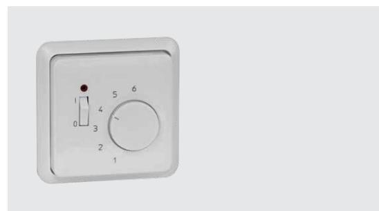
Flush-mounted, with temperature setpoint indicator, main on/off switch with indicator light, thermal feedback and additional signal input for night setback (4 K) via an external timer.
