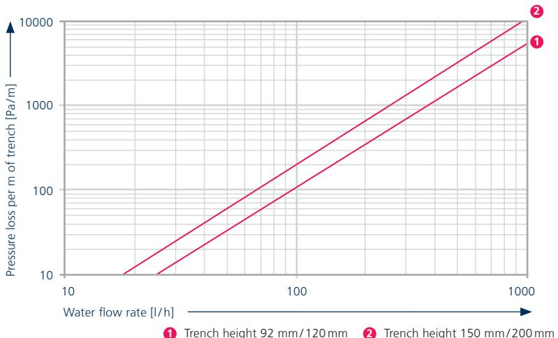
① Trench height 92 mm/120 mm    ② Trench height 150 mm/200 mm
