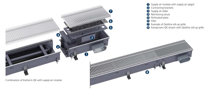
The Katherm supply air module ZL is available for all trench convectors (Katherm range). This represents a 400 mm long trench, which can be fitted to all designs of Katherm units. Treated supply air can also be fed into rooms through the Katherm supply air module ZL. This is achieved with different sizes/designs of spigots for the most diverse trench dimensions. It is possible to regulate the volumetric flow by means of slider elements in the supply air modules.
