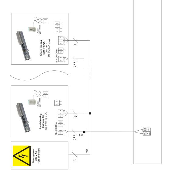
\*\* Lay shielded, paired cables, e.g. CAT5 (AWG23) of at least the same value, separately from high-voltage cables. W1: Power supply W2: Control signal for fan and actuator.
