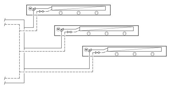
Accessories: Valve kit type 194000142110 or valve body type 194000346909, return shut-off valve type 194000145952, thermoelectric actuator type 194000146906 need to be ordered separately.
