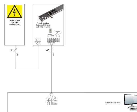
\* Lay shielded cables (e.g. IY(ST)Y, 0.8 mm), separately from high-voltage cables. W1: Power supply
