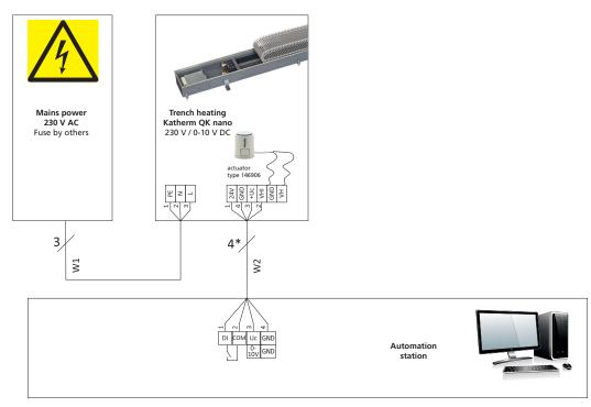
\* Lay shielded cables (e.g. IY(ST)Y, 0.8 mm), separately from high-voltage cables.
