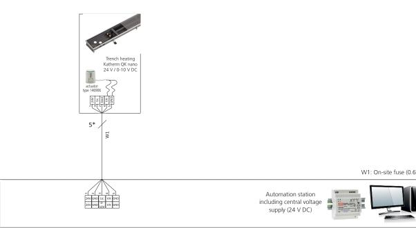
Lay shielded cables (e.g. IY(ST)Y, 0.8 mm), separately from high-voltage cables.
