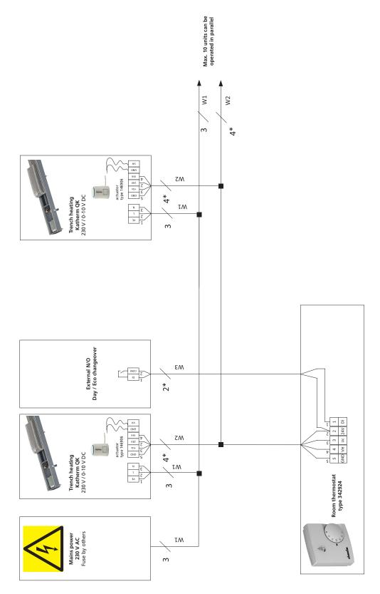
\* Lay shielded cables (e.g. IY(ST)Y, 0.8 mm), separately from high-voltage cables.
