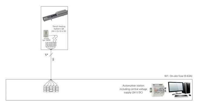
\* Lay shielded cables (e.g. IY(ST)Y, 0.8 mm), separately from high-voltage cables.
