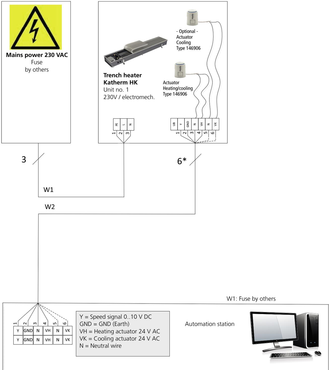
\* Lay shielded cables (e.g. IY(ST)Y, 0.8 mm), separately from high-voltage cables.
